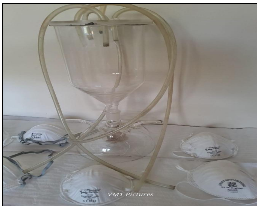
Figure 3: Dust masks combined in a dust-generating glass chamber
